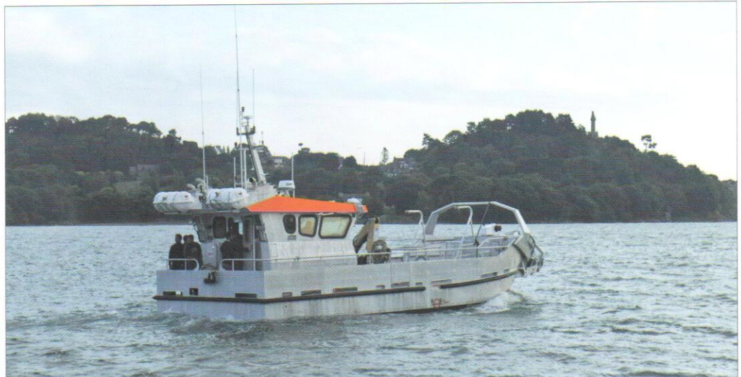
Ecoceane aluminium catamarans were designed from the start to be integrated pollution clean-up vessels.
