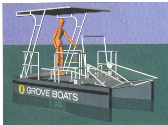
The Sea Cleaner 400 is based on an easily driven catamaran hull with the standard construction in aluminium.
