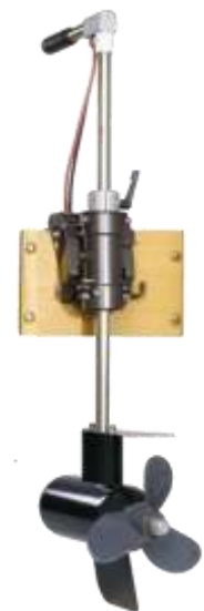
GPAV with grip for hand steering
