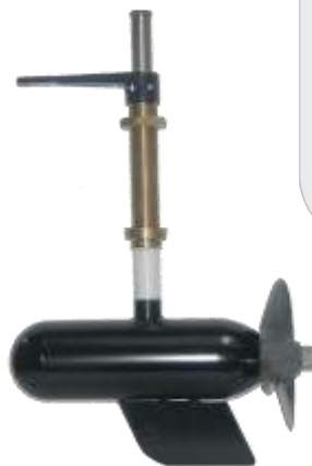
GPRV with rudder gland
