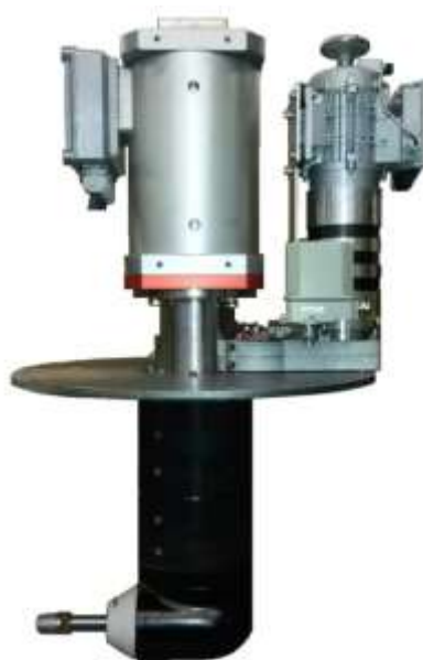
Figure: Sail-Drive electric rotatable
