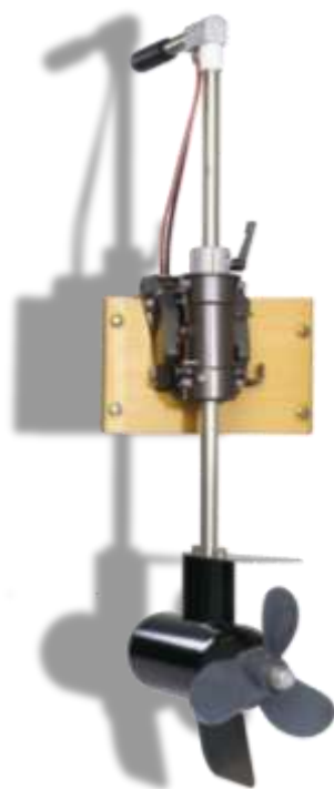
Figure: Outboarder with grip (for hand steering)
